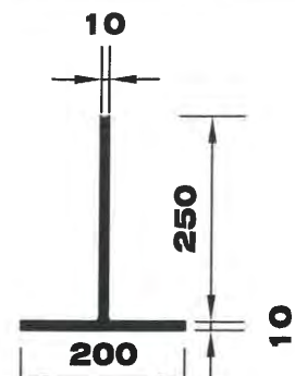
BEAM SB1 250X200X10 T section SCALE 1:10
