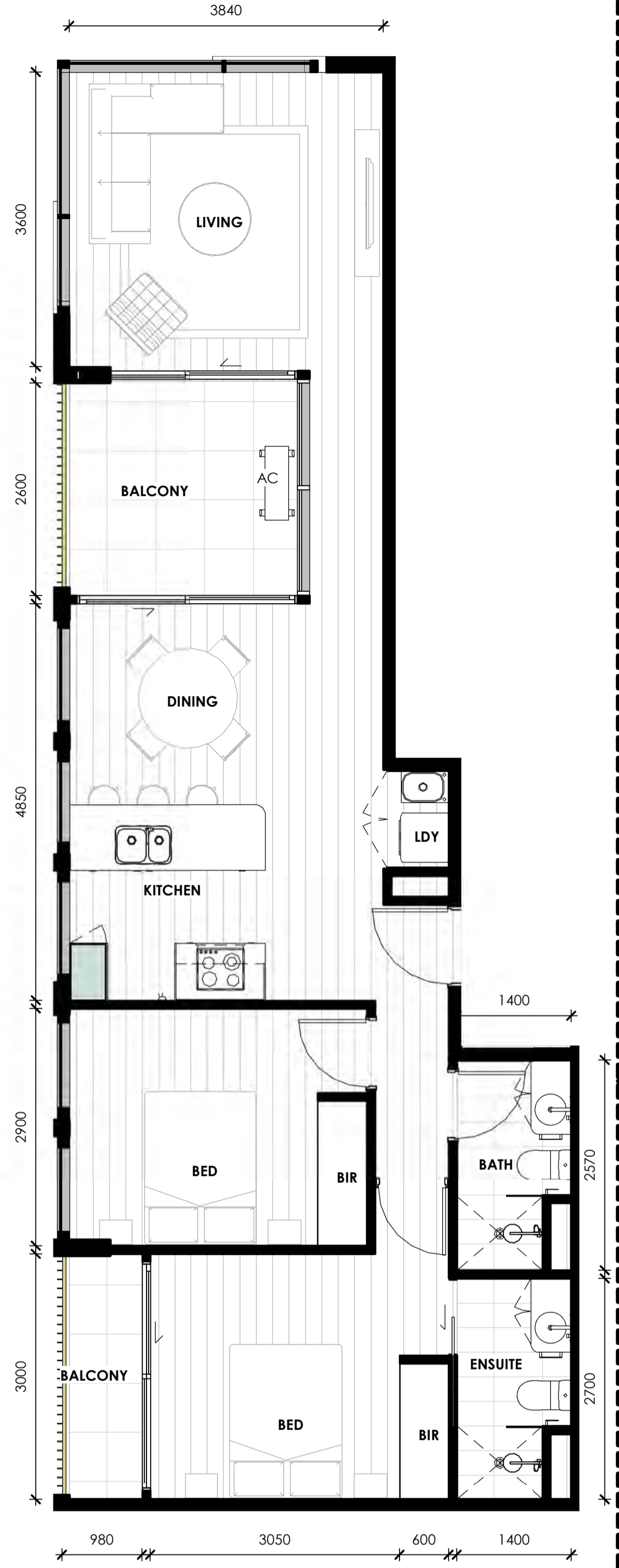
4 2 BED - TYPE 8 SCALE: 1:50 DA - UNIT SCHEDULE - 2B - T8 UNIT - TYPE GFA AREA 2B - T8 78.1M2
