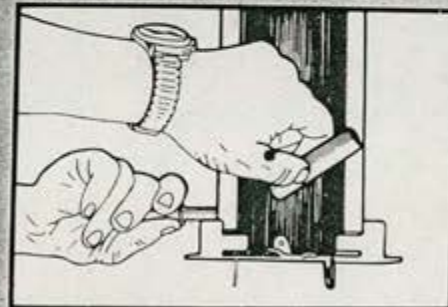
13. Place spacer (19) inside vertical support.
